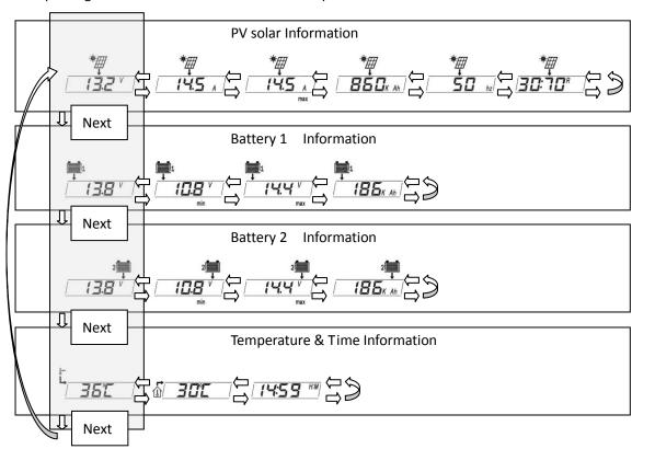
**Data setting instructions:** on reading display, press K4 for setting and next data, then save it. K1 for next data, without save. K2 and K3 for modify the data, shows as following picture 3.
